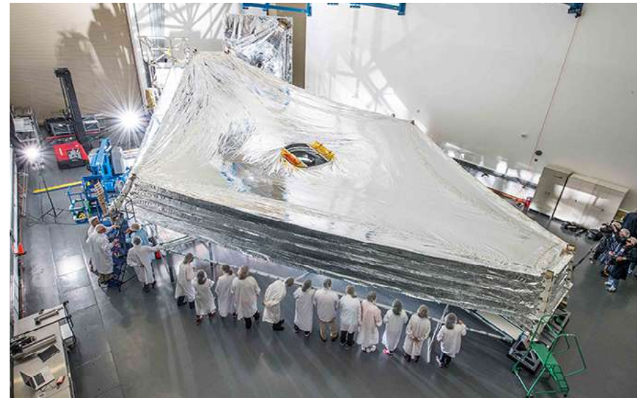
A five-layer sunshield — where each layer spans the length of a tennis court but with a thickness less than \frac{1}{10} a millimeter — protects the sensitive instruments from external heat. [NASA/Chris Gunn]
