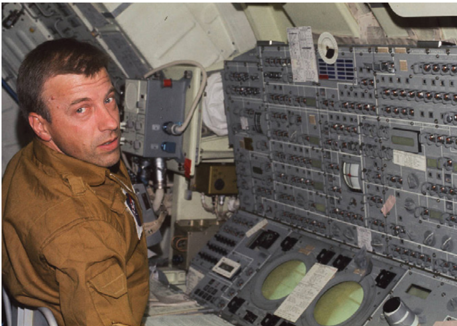
Paul J. Weitz, Skylab 2 pilot, sits at the Apollo Telescope Mount's control and display panel. [NASA]
