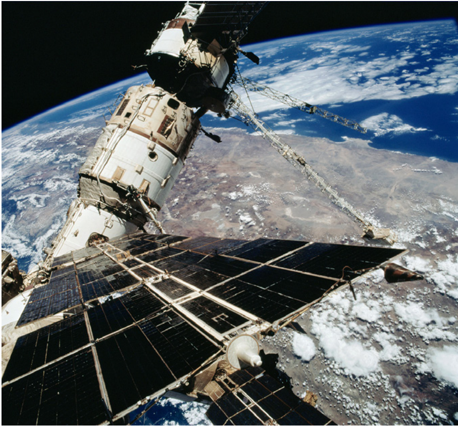
This photo, looking down one of the Mir space station's solar panels, shows a Kvant module at the diagonal. [NASA]
