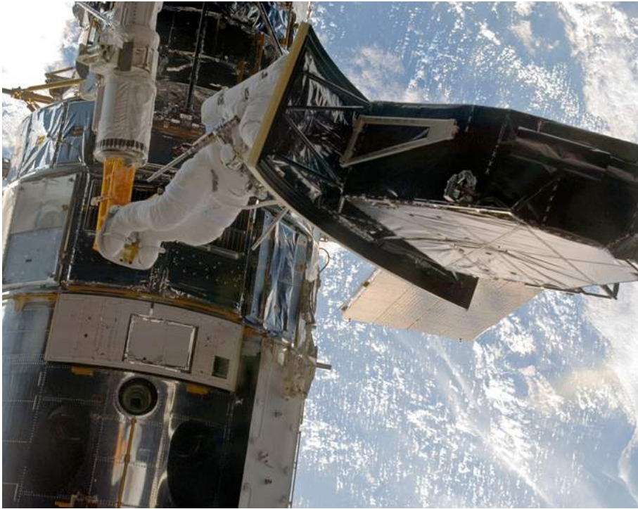
To replace the previous generation camera with the Wide Field Camera 3 during the final servicing mission, astronauts had to crank hard on a release bolt. [NASA]
