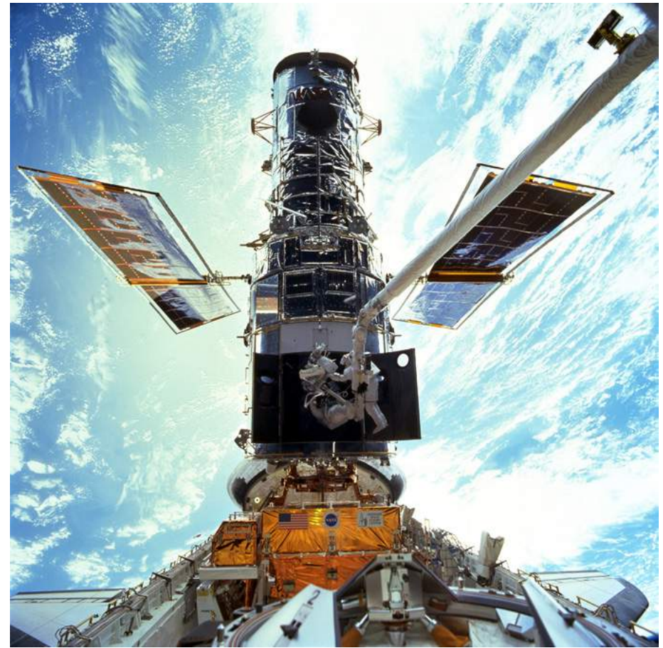
In December 1999, astronauts onboard Space Shuttle Discovery replaced the Hubble Space Telescope's main computer and the observatory's gyroscopes. Hubble wouldn't be the amazing machine it still is if it weren't for the humans involved in the decades-long project. [NASA/JSC]
