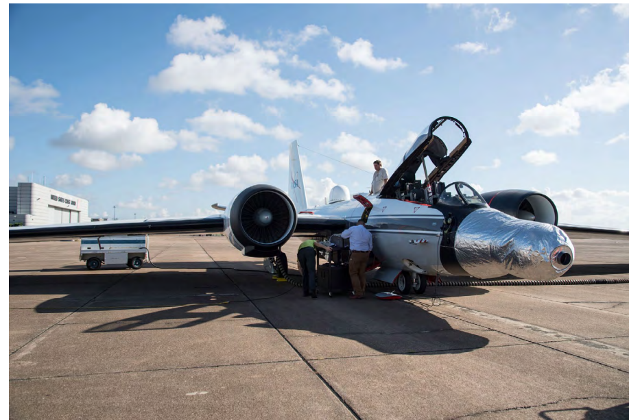
One of the WB-57F jets is readied for a test run at Ellington Field in Houston. The instruments are mounted under the silver casing on the nose of the plane and removed before flight. [NASA’s Johnson Space Center/Norah Moran]
