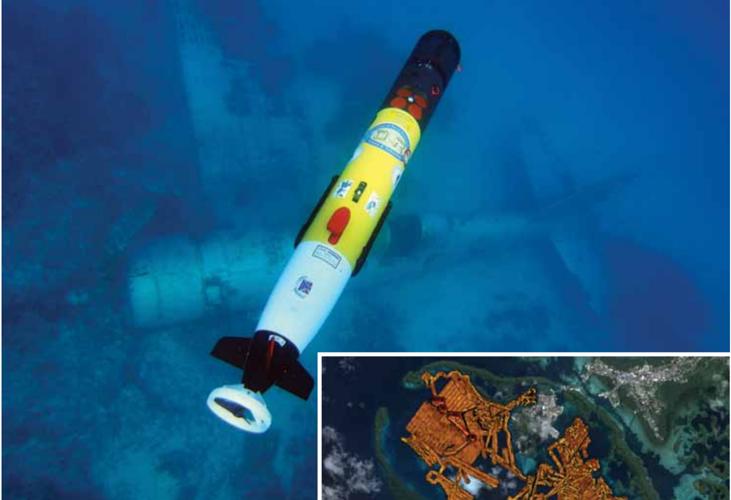
ABOVE & RIGHT A REMUS 100 AUV over an intact Corsair wreck. The inset image shows the side-scan sonar mosaic generated from multiple REMUS 100 sorties during a wide-area search. Several targets identified during this process were later examined and shown to contain aviation wreckage dating from the Second World War.
